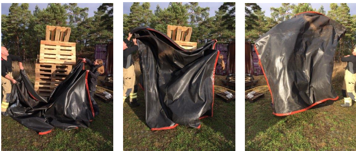
Image 6: Test how to cover a large inventory object (mock up) with a fire protective shield for two persons (Source: Norwegian Institute for Cultural Heritage Research)
