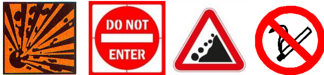
Image 15: Symbols of danger of explosions, entry forbidden, watch out for falling rubble, do not smoke (No Source)
